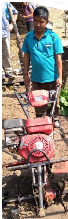
Diesel-driven mini-tractor/plough double the productivity of traditional buffalo-driven wooden ploughs
