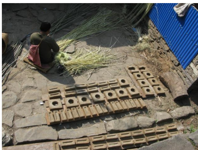
Moulded clay parts being dried before assembly of ICS
